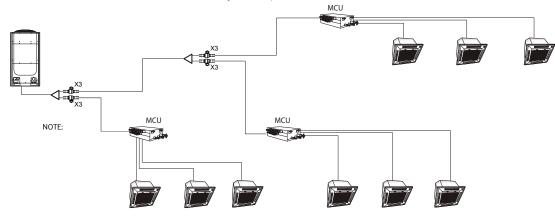
INCORRECT - Isolation valves installed immediately before MCU
